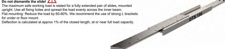
If mounting on the indirect axis, flat, as in the image above, reduce the load capacity by 60-80% and allow for increased deflection, or contact our engineers to request accurate FEA load analysis for OEM projects. We load rate per fully extended pair of slides on the direct axis, upright, with uniform loading across the beams. If load capacities need to be increased, please contact us for technical advice.
