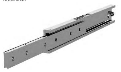
Material: All austenitic stainless steel parts Beams: Stainless 316L (1.4404) precision milled Ball bearings: Stainless 316L (1.4404) Ball cages: Stainless 316L (1.4404) End bolts & pins: Stainless A2 304 (1.4301)
