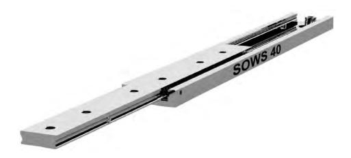
If mounting on the indirect axis, flat, as in the image above, reduce the load capacity by 60-80% and allow for increased deflection, or contact our engineers to request accurate FEA load analysis for OEM projects. We load rate per fully extended pair of slides on the direct axis, upright, with uniform loading across the beams. If load capacities need to be increased, please contact us for technical advice.
