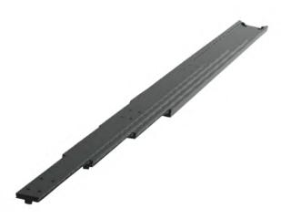
If mounting on the indirect axis, flat, as in the image above, reduce the load capacity by 60-80% and allow for increased deflection, or contact our engineers to request accurate FEA load analysis for OEM projects. We load rate per fully extended pair of slides on the direct axis, upright, with uniform loading across the beams. If load capacities need to be increased, please contact us for technical advice.
