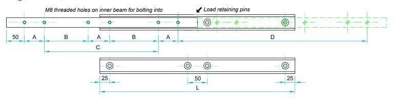
Full traversing is 1 x D when the slide is mounted in the open position. Single extension is 0.5 x D
