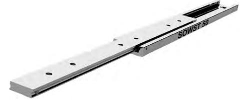
If mounting on the indirect axis, flat, as in the image above, reduce the load capacity by 60-80% and allow for increased deflection, or contact our engineers to request accurate FEA load analysis for OEM projects. We load rate per fully extended pair of slides on the direct axis, upright, with uniform loading across the beams. If load capacities need to be increased, please contact us for technical advice.
