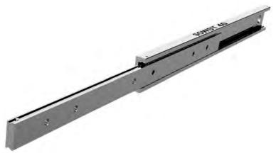
Material: All austenitic stainless steel parts Beams: Stainless 316L (1.4404) precision milled Ball bearings: Stainless 316L (1.4404) Ball cages: Stainless 316L (1.4404) End bolts & stopping pins: Stainless A2 304 (1.4301) Surface treatment: Polished
