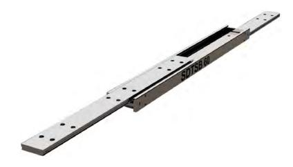
If mounting on the indirect axis, flat, as in the image above, reduce the load capacity by 60-80% and allow for increased deflection, or contact our engineers to request accurate FEA load analysis for OEM projects. We load rate per fully extended pair of slides on the direct axis, upright, with uniform loading across the beams. If load capacities need to be increased, please contact us for technical advice.
