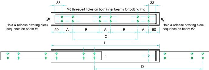
Full traversing is  $2 \times D$  when the slide is mounted in the open position
