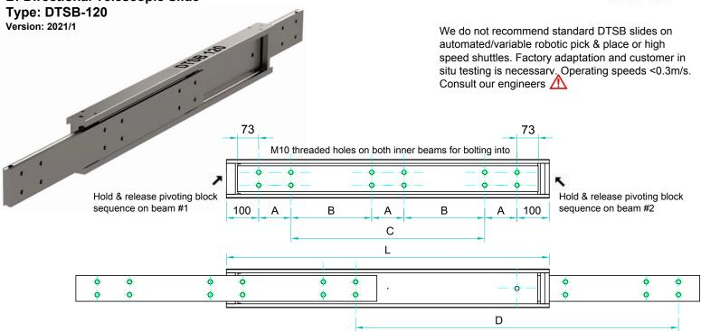
Full traversing is 2 x D when the slide is mounted in the open position
