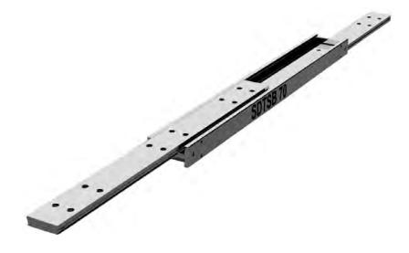
If mounting on the indirect axis, flat, as in the image above, reduce the load capacity by 60-80% and allow for increased deflection, or contact our engineers to request accurate FEA load analysis for OEM projects. We load rate per fully extended pair of slides on the direct axis, upright, with uniform loading across the beams. If load capacities need to be increased, please contact us for technical advice.
