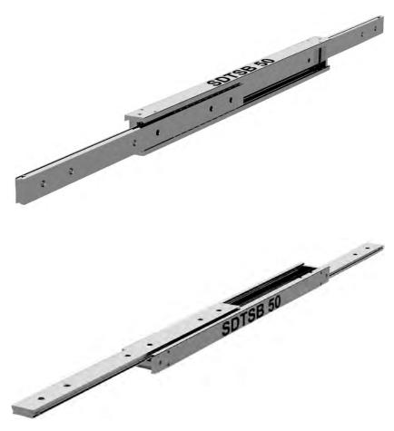
If mounting on the indirect axis, flat, as in the image above, reduce the load capacity by 60-80% and allow for increased deflection, or contact our engineers to request accurate FEA load analysis for OEM projects. We load rate per fully extended pair of slides on the direct axis, upright, with uniform loading across the beams. If load capacities need to be increased, please contact us for technical advice.
