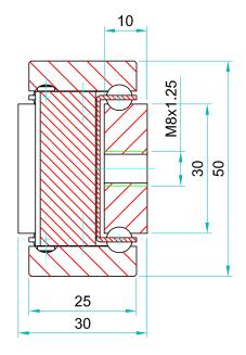
We do not recommend standard DTSB slides on automated/variable robotic pick & place or high speed shuttles. Factory adaptation and customer in situ testing is necessary. Operating speeds <0.3m/s. Consult our engineers
