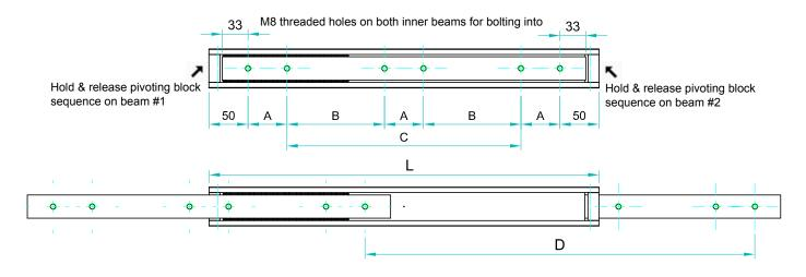
Full traversing is 2 x D when the slide is mounted in the open position
