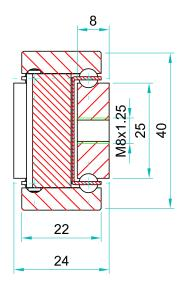
We do not recommend standard DTSB slides on automated/variable robotic pick & place or high speed shuttles. Factory adaptation and customer in situ testing is necessary. Operating speeds <0.3m/s. Consult our engineers
