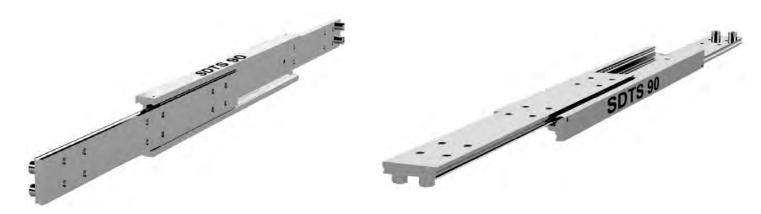
If mounting on the indirect axis, flat, as in the image above, reduce the load capacity by 60-80% and allow for increased deflection, or contact our engineers to request accurate FEA load analysis for OEM projects. We load rate per fully extended pair of slides on the direct axis, upright, with uniform loading across the beams. If load capacities need to be increased, please contact us for technical advice.
