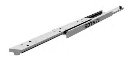
If mounting on the indirect axis, flat, as in the image above, reduce the load capacity by 60-80% and allow for increased deflection, or contact our engineers to request accurate FEA load analysis for OEM projects. We load rate per fully extended pair of slides on the direct axis, upright, with uniform loading across the beams. If load capacities need to be increased, please contact us for technical advice.
