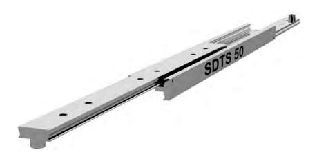
If mounting on the indirect axis, flat, as in the image above, reduce the load capacity by 60-80% and allow for increased deflection, or contact our engineers to request accurate FEA load analysis for OEM projects. We load rate per fully extended pair of slides on the direct axis, upright, with uniform loading across the beams. If load capacities need to be increased, please contact us for technical advice.
