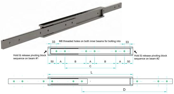
Full traversing is 2 x D when the slide is mounted in the open position
