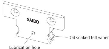
The plastic lubrication covers contain oil soaked felt wiper which can be re-lubricated via lubrication holes shown above.
