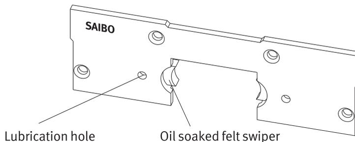
The plastic lubrication covers contain oil soaked felt wiper which can be re-lubricated via lubrication holes shown above. These lubrication covers will require re-lubrication regularly dependent on the application requirements
