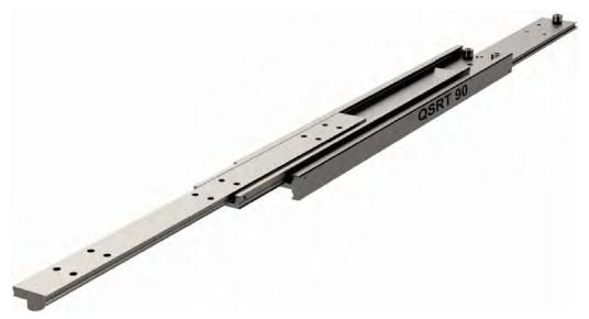
If mounting on the indirect axis, flat, as in the image above, reduce the load capacity by 60-80% and allow for increased deflection, or contact our engineers to request accurate FEA load analysis for OEM projects. We load rate per fully extended pair of slides on the direct axis, upright, with uniform loading across the beams. If load capacities need to be increased, please contact us for technical advice.
